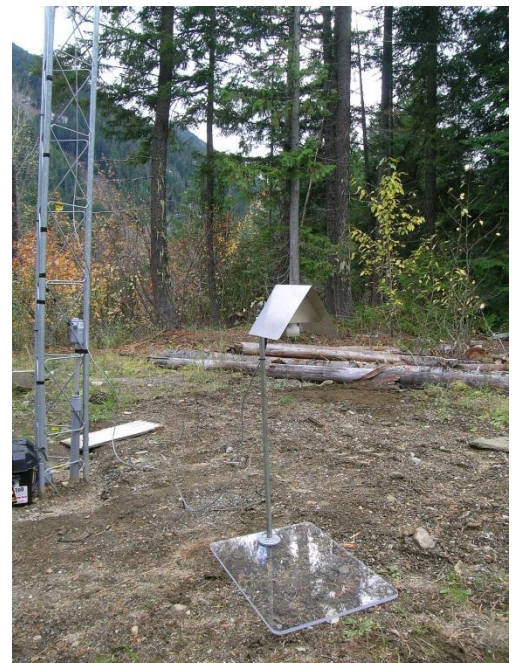
Figure 31. 24-hr depth sensor with hat—installed adjacent to Berne weather tower supporting AT, RH, precipitation gage, total depth sensor and datalogger/modem enclosure.
