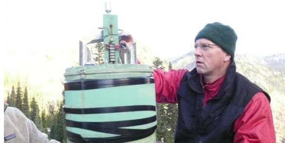
Figure 29. Kenny working on the Chinook Pass precipitation gage...clipped in at the top of a 30 ft tower.
