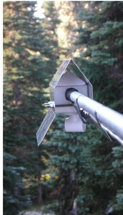
Figure 28. Depth gage hats at both Chinook Pass and Sunrise that help prevent snow accumulations from creeping over the sensor and preventing measurement.
