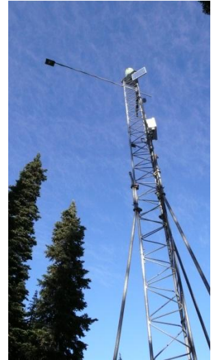
Figure 30. The 30 ft Chinook Pass base station tower with supporting struts, datalogger enclosure, RF antenna, total depth sensor, and precip gage on top.
